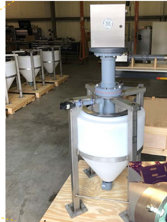
Sulfite Analyzer and sample sink
